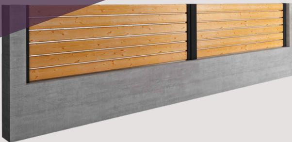
150mm x 30mm planks with a 70 x 70mm internal tubular post & 80 x 50mm external tubular post
